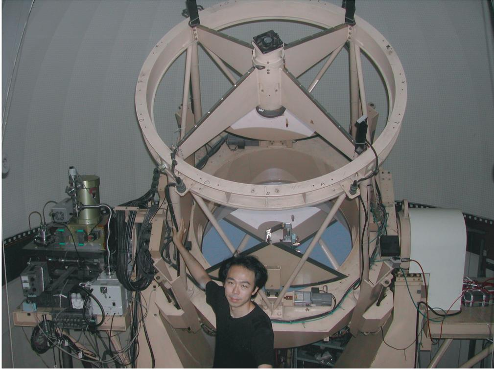
**Figure 1.** A 1.3 m diameter telescope at the roof top of ISAS, viewing down from the top. The mechanically cooled near infrared detection system is mounted on the Nasmyth table at the left side of this picture. One of the coauthors, D. Yonetoku is standing in front of the telescope. More details of specification of this telescope are shown in the table and also in the attached pictures in each section.
