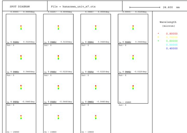
**Figure 4.** A ray trace simulation to check the quality of focus inserting this grism into a conversion ray of the Cassegrain focus. The figure shows a image quality of dispersion in 600, 700 and 800 nm for several different incident angles.
