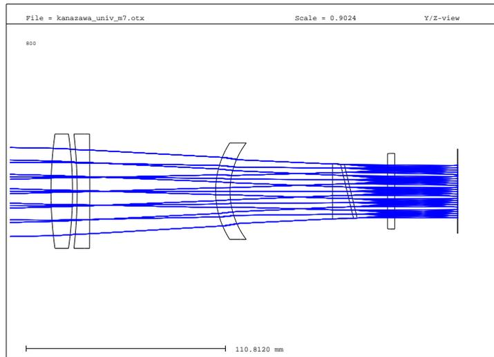
**Figure 3.** A ray trace simulation to check the quality of focus inserting this grism into a conversion-ray of the Cassegrain focus. The first achromatic lens and the second non-spherical lens are used for a wider FOV. The last flat glass is for an adjustment of the focal length to the case of without the grism.
