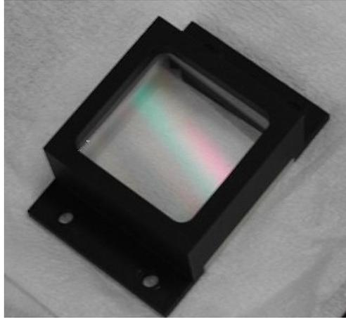
**Figure 2.** A grism designed for the 1.3 m telescope R band. The number of rule is 200 lines per mm and the size of the grism is 33 x 33 mm and 13.5 mm in thickness. This was inserted into the conversion-ray of the Cassegrain focus.
