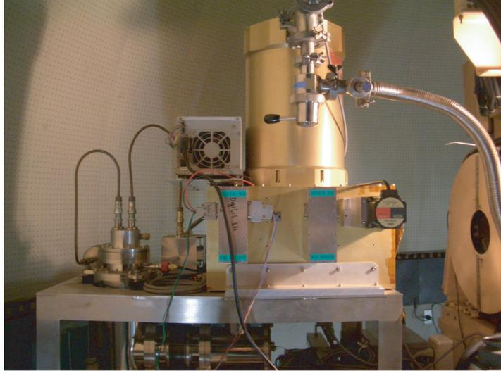
**Figure 6.** A vacuum chamber of the IR Lab. is used for installing the NICMOS (CdHgTe) chip with 256x256 pixels. At the right side of the picture, a mechanical refrigerator, which is connected to the vacuum chamber beneath the chamber, is mounted to keep this system 70K. The Nasmyth hole is seen at the right side of the picture. A stepping motor to control the three filters of J, H and Ks is also seen on the right corner of the vacuum chamber
