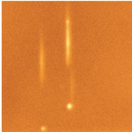
**Figure 5.** A dispersive image of 3C273 by the grism, mounted on the path of Cassegrain focus. A 0-th order image of the 12.8 magnitude QSO: 3C273 and the dispersive image is seen in the center. The Hydrogen  $\alpha$  and  $\beta$  are clearly seen. Refer to the 0-th order spots, we can calibrate the wavelength.
